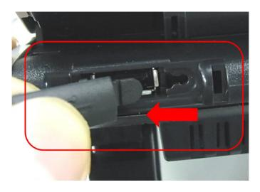
**Note:** Do not pull the cover upward. If the USB Port Cover is pulled upward, the cover may rip apart from the connector.
