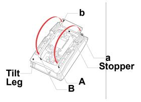
While pushing the two hooks, slide the tilt leg downward. Remove the tilt leg from the terminal.
