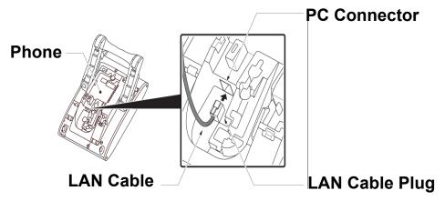
2 Thread the LAN cable through the groove on the back of the phone.
