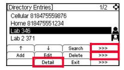
This displays the name and number for the entry, along with the Speed Dial and Monitor settings.
