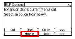
You can then press the Barge or Record soft key to barge on the call or start a recording of the call. Press Exit to exit this screen without starting a Barge session or recording of the call.
