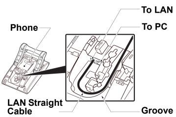
3 If you have not connected the DT700 phone to a PoE jack, connect the AC/DC adapter to the phone as shown below.
