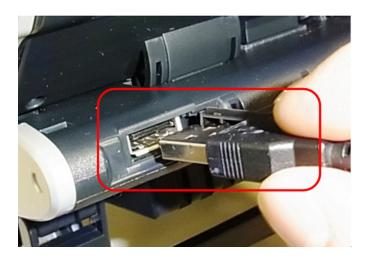
Make sure you are inserting the plug with the correct orientation, and push the USB connector into the port until it stops.
