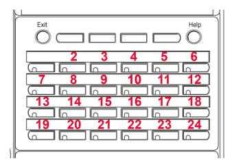
Figure 8.16 DT730 (ITL-12D), DT730G (ITL-12CG) and DT730G (ITL-12DG) Speed Dial Key Numbering
