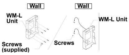
When attaching wall mount unit to the wall plate:
