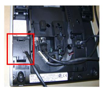
5 Connect the network cable end of the Jabra EHS Adapter to the AUX port AUX on the back of the headset base station.
