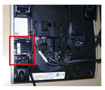
3 Connect the 10 pin connector of the Jabra EHS Adapter to the SIDE 2 port on the back of the phone.
