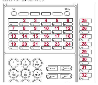
Figure 8.15 DT730 (ITL-24D), DT730G (ITL-24CG), and DT730G (ITL-24DG) Speed Dial Key Numbering
