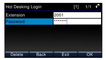
The Hot Desking Extension field has focus when entering the Hot Desking Login page, and the keypad is in numeric entry mode.
