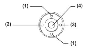
Up/Down Keys Used to adjust various volume levels. (1) • Handset, Speaker and Headset volume: Press (UP) or (DOWN) key during conversa-• Ring Volume: Press (UP) or (DOWN) while on hook. · Soft Ring Volume: Press (UP) or (DOWN) key while Soft Ring is playing. (2) Redial Key Pressing this key redials the last number dialed.
