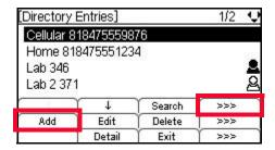
3 Use the telephone keypad to enter the name and press Enter on the cursor pad or the OK softkey.
