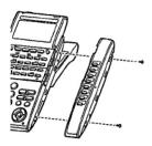
On the back of the phone, press the tab on the port cover on the left side of the back of the phone to release the protective cover that is over the ports. Remove the cover.
