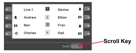
The Page Icon indicates the currently displayed page. You can change pages using the Scroll key. The display offers the following Programmable Keys on the four pages available on the display:
