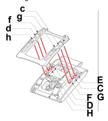
Fit the indicated portions (a and b) of the stopper into grooves (A and B) on the tilt leg.
