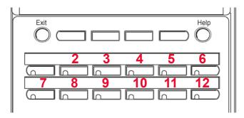
Figure 8.17 DT710 (ITL-6DE) Speed Dial Key Numbering
